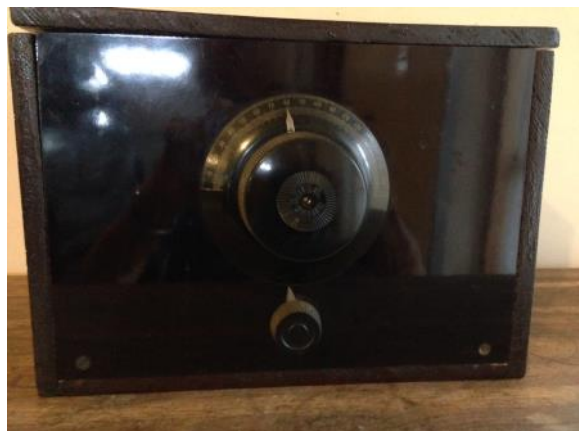
Homebrew One Tube Receiver
