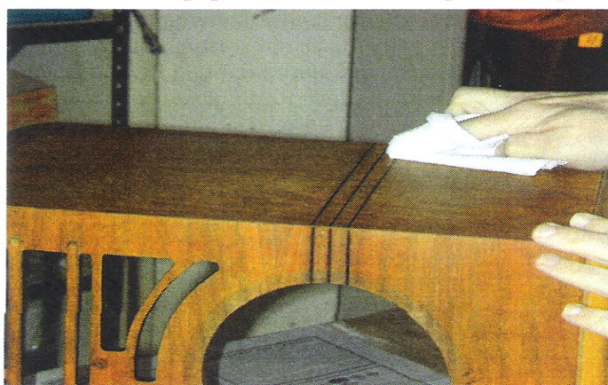
Fig13: Cleaning slop over from the groove edges.
