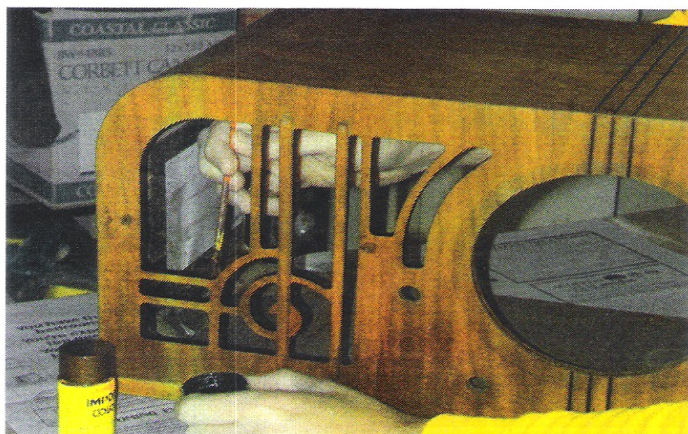
Fig12: Coloring edge of the speaker grill opening.
