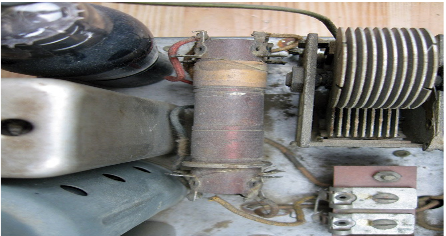
The other two oscillator coils sharing a common coil form on top of the chassis
