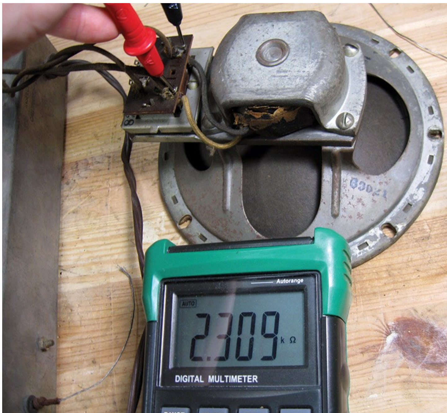
Checking the speaker field coil resistance; 2,309 ohms
