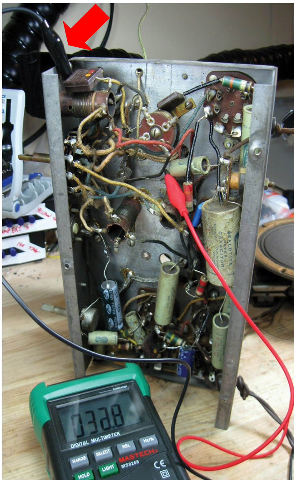
Measuring the primaries of the antenna coils
