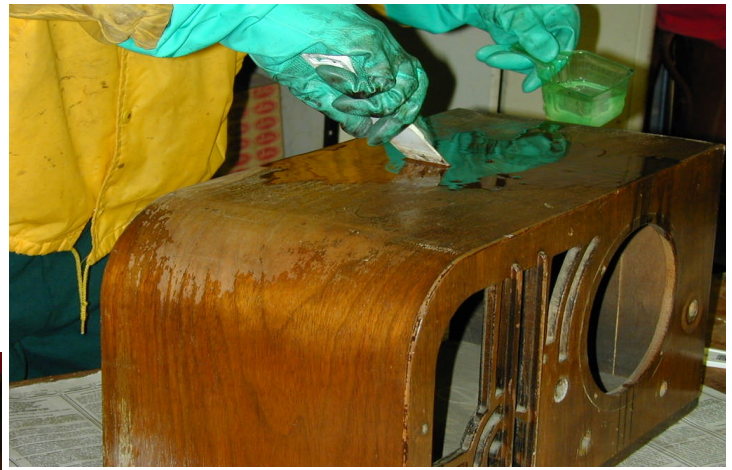
Figure 8: Scraping the softened old finish
