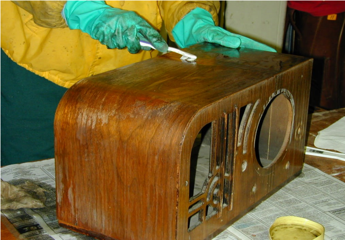
Figure 9: Using an old toothbrush for details
